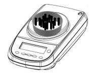
10. As soon as it is reached a sufficient number of pieces, this number is displayed and it will be possible to go on with count by loading the pieces count on the balance pan.
